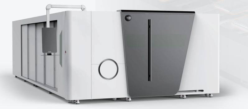
tacle avoid system BodorGenius uses sensors and algorithms to detect potential obstacles like tilting parts and automatically ds a potential collision.
