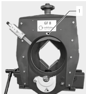
Position of the safety screw for the GF 8, GF 12 (AVM/MVM).
