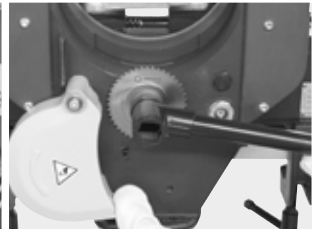
Fixture for saw blade/bevel cutter
