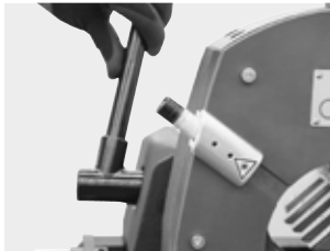
Fixture for clamping jaws (GF 4 (AVM/MVM) only)
